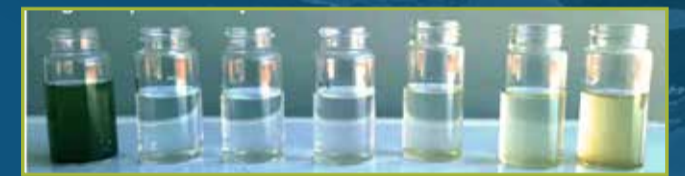
Two fermented products (far left) and increasing treatment concentrate. from left to right: 0.1, 0.25, 0.5, 1.0, 2.0, and 5.0 g/L
